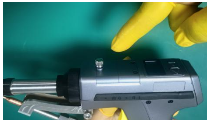
① Unscrew the protective lens screw
