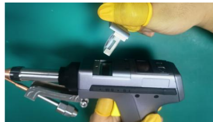
② Remove the protective lens holder
